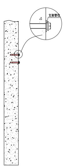
Step two: Lock the explosive screw: drive 12mmx65mm explosive screw into the mounting holes and tighten with it with a wrench.
