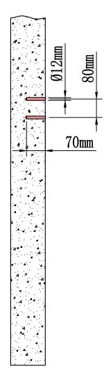
Step one: Drill the installation holes: drill 12mm in diameter and 70mm in length according to the marked dimension.
